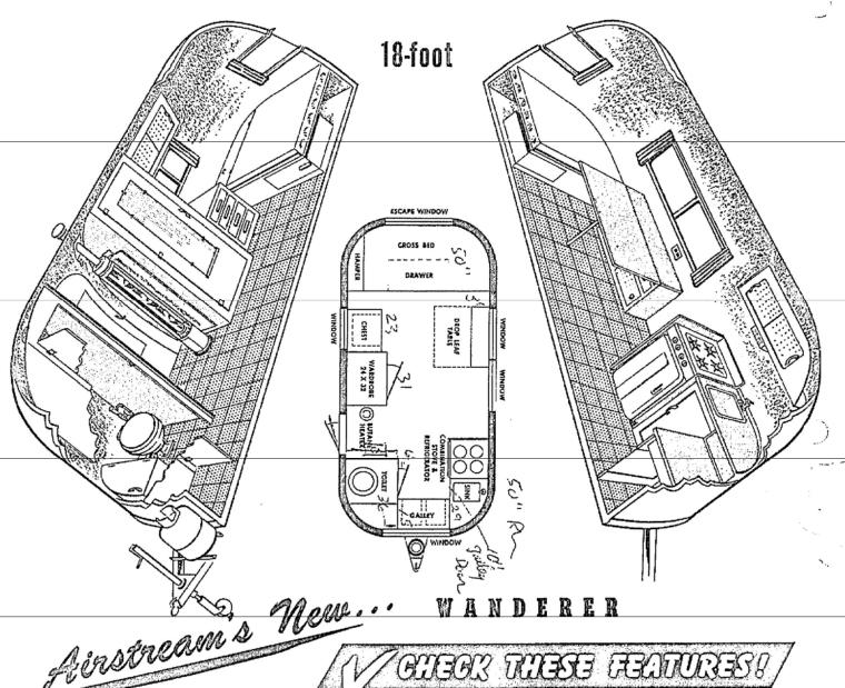
Overall length -13 ft. Body length - 15 it. Overall weight - 2,130 lbs. Hitch weight - 270 lbs. 43" cross bed.
