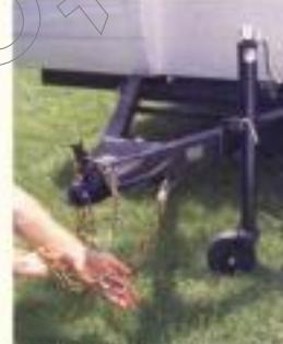
not interfere with tow vehicle's tailgate or rear mounted spare tire. (Highlander Series features center mount jack.) Safety lock chains provide a positive locking connection between the trailer and tow vehicle.
