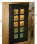
The Intellitec Multiplex Lighting System with memory is accessible from four locations throughout the DynaQuest XL. This convenient system allows the user to completely shut down all of the 12-Volt lighting, from ceiling to floor, by holding one button down for a few seconds. Controls are located in the overhead console cab area, entry door, bathroom (near the vanity sink), and in the bedroom overhead cabinet.
