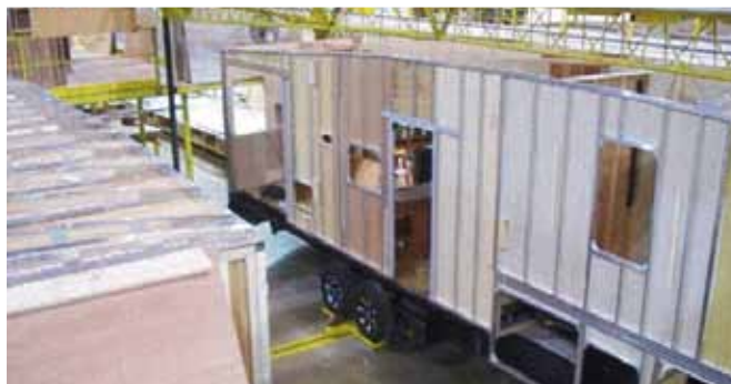
ALUMINUM STUDDED SIDEWALLS AND ROOF TRUSSES ON 16" CENTERS OR LESS
