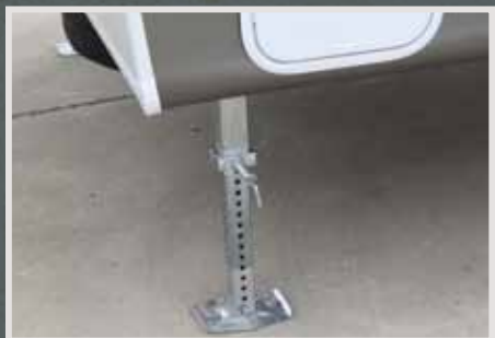
Wide stance power front jacks with quick release snap pins.
