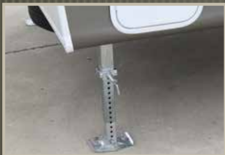
Wide stance power front jacks with quick release snap pins. (Fifth wheels)
