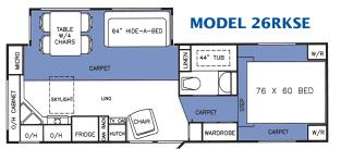
Pry Weight 3673 kg/8095 lbs. Hitch Weight 592 kg/1305 lbs. Net Carrying Capacity 862 kg/1900 lbs.
