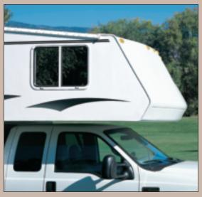
Molded fiberglass front caps are aerodynamically designed to eliminate wind resistance and provide protection against rock damage. Bedrooms have superior headroom not found in other campers.
