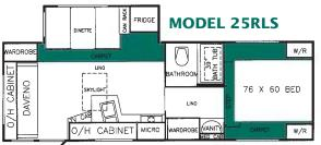
Dry Weight 3344 kg/7370 lbs. Hitch Weight 603 kg/1330 lbs. Net Carrying Capacity 740 kg/1630 lbs
