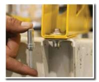
Huck fasteners can't be over or under tightened ensuring the strongest and longest lasting connection of the truss system to the chassis.
