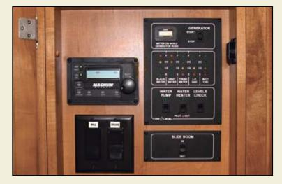
CONTROL PANELS AND SWITCH BANKS ARE PLACED IN A CENTRALIZED AREA. NO MORE RUNNING FROM SWITCH TO SWITCH WHEN YOUR READY TO LEAVE OR WISH TO KNOW THE STATUS OF YOUR WATER, WASTEWATER, LP OR BATTERY POWER LEVELS.
