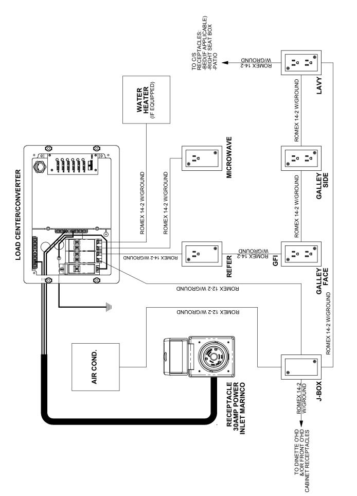
**120 VOLT CIRCUITS WIRING**
