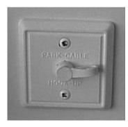
The park cable inlet is located on the roadside of the trailer. This allows for the connection from campground cable service via a coax cable (not provided) to the trailer. The cable inside the trailer is terminated at the primary TV location at a wall plate. If your trailer is also equipped with a TV antenna, the park cable terminates into the TV outlet. With the switch in the "OFF" position, the park cable signal is sent through the outlet.
