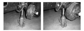
Place a hydraulic jack on a level surface under the lower lip of the axle of which the tire being changed is located. Do not locate the jack along the frame rail as this could cause damage to the frame rail.
