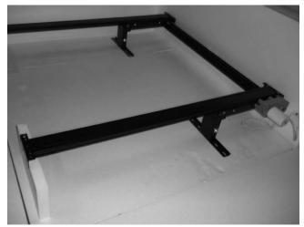
The slide-out room uses a rack and pinion mechanism to move the room. The pinion gears are driven by a 12-volt DC electric motor by the trailer battery(s). A switch mounted on the wall controls the room movement.
