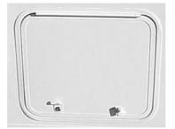
Various exterior compartment doors provide access to certain appliances, controls, and general storage. Exterior compartment doors may not be water tight in all weather and road conditions. Any article which could be damaged by water or dirt should be carried inside the trailer or tow vehicle.
