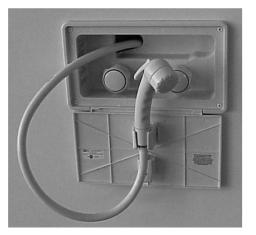
The exterior wash station is located in the service center on the roadside compartment for exterior use. It uses water from the fresh water tank or when connected to the city water hookup. The showerhead is equipped with a flow control to allow you to conserve water. This flow control is not a permanent shut off.
