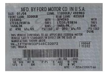
A Federal Certification Label is required by law on all motor vehicles. On tow vehicles it is usually located on the driver side door post. It lists the Gross Vehicle Weight Rating (GVWR), the maximum weight at which the vehicle may be operated. It also provides a Gross Axle Weight Rating (GAWR), the maximum weight allowed for each axle.
