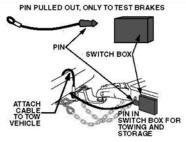
If the coupler or hitch fails, a properly connected and working breakaway switch will apply electric brakes on the trailer. The safety chains will keep the tow vehicle attached and as the brakes are applied at the trailer's axles, the trailer/tow vehicle combination will come to a controlled stop.
