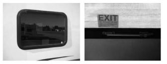
Read and understand these instructions before you need to use them. The emergency exit window provides an escape route in case the trailer must be evacuated under emergency conditions and the path to the main entry door is blocked.
