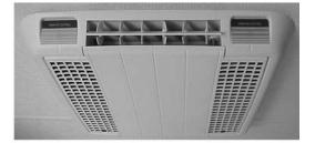
The roof-mounted Air Conditioner operates on 120volt power, which is supplied through the 30-amp power cord, either from an outside 120-volt power service or by the onboard generator, if equipped.
