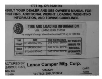
The second (middle) label is the Tire and Loading Information Tag. It lists the trailer VIN number and maximum cargo capacity of the trailer as equipped by Lance. It also lists the tire size and Cold Tire Pressure of the tires that are supplied on your trailer.
