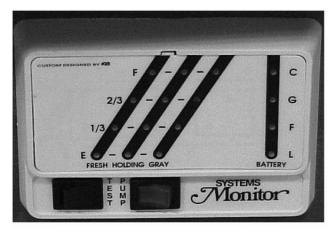
The systems monitor panel incorporates controls for the water and holding tank levels, battery condition and water pump. It may also control the water heater.
