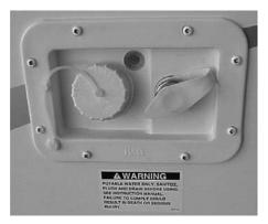
The city water inlet connection is located under the roadside overhang.
