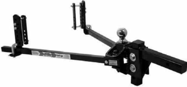
**Tongue weight on a bumper pull trailer should be 10-15% of the total weight of the trailer plus cargo (Gross Vehicle Weight, or “GVW”). The tongue weight on a 5th Wheel trailer should be 20-25%.**
