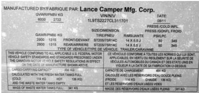
The second (lower) label is the Federal Certification Tag. It contains the Manufacturer's Name, VIN number, month and year built, GVWR, GAWR of each axle, and the tire size, rim size and PSI.
