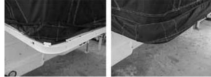
Grab the tent flap along the bed door and pull it over the edge of the door. From the inside of the tent, connect the tension bar into the tent bow and lock into position.
