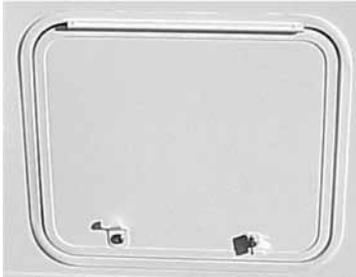
Various exterior compartment doors provide access to certain appliances, controls, and general storage. Exterior compartment doors may not be water tight in all weather and road conditions. Any article which could be damaged by water or dirt should be carried inside the trailer or tow vehicle.
