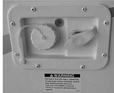
The fresh water system should be sanitized at the initial filling, after a period of storage or if contaminated. See "Sanitize Fresh Water System" in this section. Fill tank slowly. Do not overfill. Do not leave unattended while filling. Structure damage may occur.
