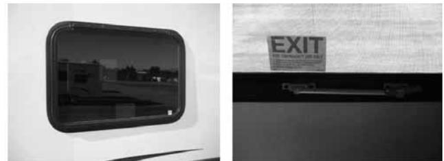
The emergency exit window is identified by the red handle(s) and EXIT label.
