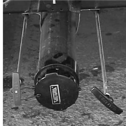
The holding tanks terminate in a valve arrangement that permits each tank to be dumped separately or together. The valves are called “knife valves”. A blade closes the opening in the sewer drain pipes. The blade is connected to an extension handle that is pulled to release the contents of the tank(s).
