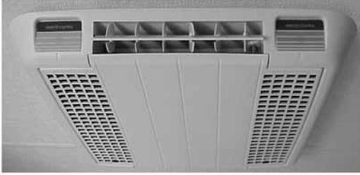
The roof-mounted Air Conditioner operates on 120-volt power, which is supplied through the 30-amp power cord, either from an outside 120-volt power service or by the onboard generator, if equipped.
