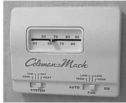
The wall-mounted combination thermostat will operate either the furnace or air conditioner from one location.
