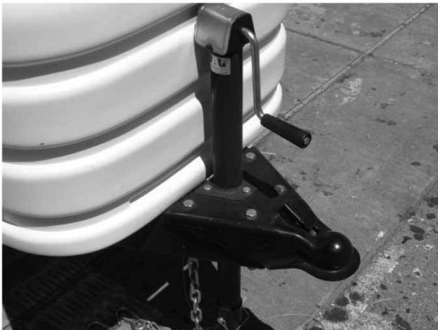
The ball hitch trailer is fitted with a tongue jack that can raise and lower the coupler. The tongue jack is mounted to the A-frame part of the trailer. By rotating the jack handle clockwise, the jack will extend and raise the tongue of the trailer.
