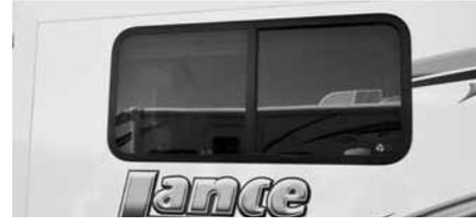
Windows in your trailer are slider or torque pane style. Open slider windows by rotating the locking lever and sliding the window. Open torque windows by turning the crank located at the bottom of the window frame, clockwise to open, counterclockwise to close.
