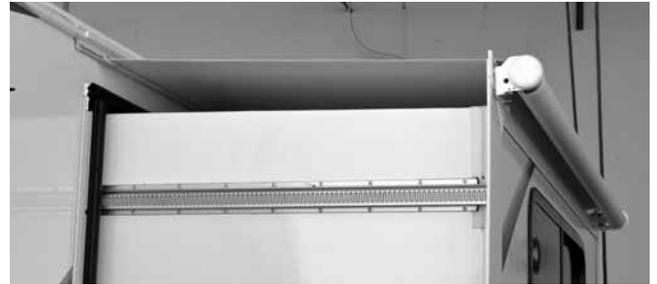
The slideout cover extends and retracts with the slide room. It helps to divert water off the slide room roof and helps in keeping the roof clean of debris. The room seal can become less effective or even damaged if the slide room roof is not kept clean.
