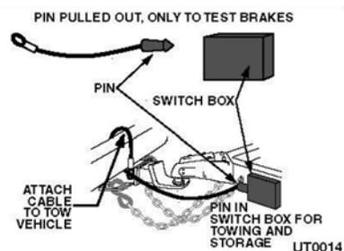
If the coupler or hitch fails, a properly connected and working breakaway switch will apply electric brakes on the trailer. The safety chains will keep the tow
