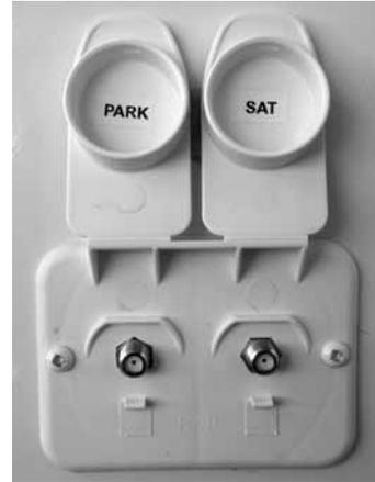
The park/sat dish inlets are located on the driver's side of the trailer. The park cable inlet allows for the connection from the campground cable service to the trailer. The satellite inlet allows for the connection from a portable dish. Both cables terminate inside the camper at the primary TV location in a wall plate. The park cable is connected to the 12-volt/TV outlet. With the switch on the outlet in the "OFF" position, the park cable signal is sent through the outlet.
