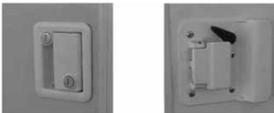
The entry door lock and deadbolt are keyed alike. The key is double sided so it can be installed into the lock either direction. Be sure to write down the key number on the Identification Information Page located in the front of this manual. Your Lance Dealer can obtain duplicates with this number.
