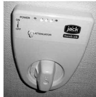
The roof-mounted HDTV antenna is designed for reception of digital signals, as well as UHF and VHF channels. Consult the manufacturer's operation instructions for proper use. The TV jack outlet is located at the primary TV location. If you are dry camping, the booster switch should be turned "OFF" when not viewing the TV to prevent battery drain as the indica-
