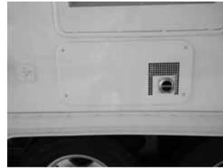
The furnace is a forced air unit fueled by propane and electronically powered by 12-volts. A wall-mounted thermostat similar to those used in homes controls it. To start the furnace, set thermostat switch to the ON position and set desired temperature. The furnace will cycle on and off as needed. To stop the furnace, set the thermostat to lowest setting and the OFF position. If your furnace does not operate properly, check the battery condition and propane supply.
