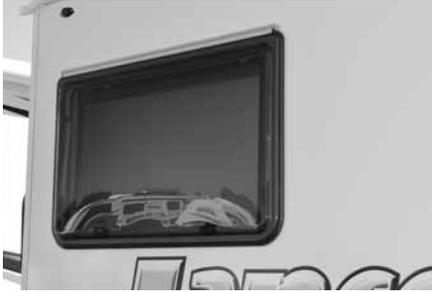
Your trailer may be equipped with “Lightweight” Acrylic Windows. To open this style of window, locate the locking lever(s) located at each side and at the bottom of the window. Rotate the lever to un-lock the window. There are struts located at each vertical pillar of the window which retain the window at the desired open position. To close the window, simply raise the window slightly and return the window to the closed position and rotate the levers to the locked position.
