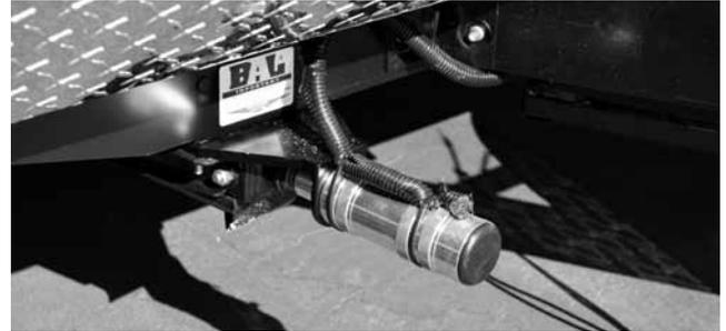
Your trailer may be equipped with electric stabilizer jacks. The control panel is located in the forward driver side storage compartment. The control panel is made up of four (4) control switches that enable independent operation of each jack and a system kill switch. To operate the leveling system, ensure the 12-volt source is activated, extend and/or retract each jack using the control switch(s).
