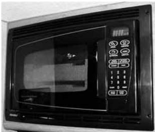
Please read all instructions that come with the convection or microwave oven before use. The oven should never be operated empty. When operating on your generator (if equipped) power is limited. If the roof air conditioner is operating there may not be enough power to operate the microwave.
