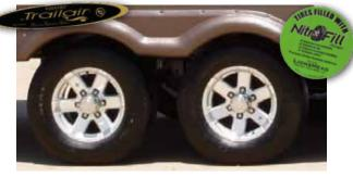
■ Nitrogen filled tires are standard on all Raven models. Also standard is a rubberized Equa-Flex Trailair® suspension system. Aluminum wheels are optional.
