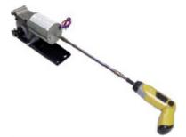
4. If the cables tighten, and the motor is difficult to turn, REVERSE THE DIRECTION. Over-torquing can happen, resulting in severe damage.
