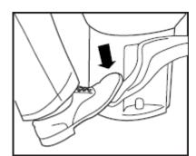
To flush the foot pedal style, depress the pedal all the way until rinse clears the bowl. Be sure to release the lever slowly. Movement of the flush lever opens the waste valve and allows the water to pass into the holding tank.
