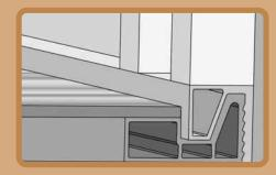
Interlocking Floor-To-Sidewall Construction locks tightly to keep out water, dust and noise, and helps eliminate squeaks and rattles.
