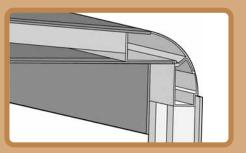
Interlocking Ceiling-To-Sidewall Construction helps keep the box square. This assures a proper cabinet fit.
