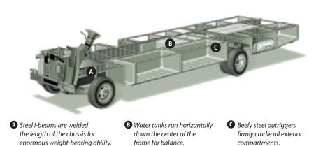
Drawing for illustrative purpose only to highlight aspects of motor home construction. Actual motor home design depends on model and is subject to change.
