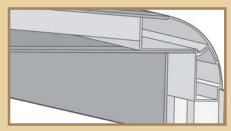
INTERLOCKING CEILING-TO-SIDEWALL CONSTRUCTION helps keep the box square. This assures a proper cabinet fit.
