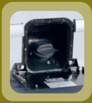
**THE FUEL FILL** is located in the back, so you can pull into any pump at the filling station and refuel (select models).
