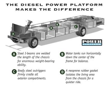
Drawing is for illustrative purpose only to highlight aspects of motor home construction. Actual motor home design depends on model and is subject to change.
