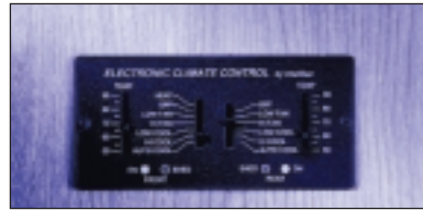
An optional electronic climate control system with dual A/C controls enables a separate climate in the front and rear of the coach.
