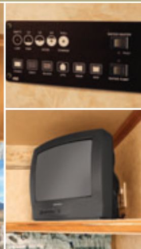
THE SYSTEM MONITOR PANEL provides a central place to conveniently check all of your holding tank levels.
