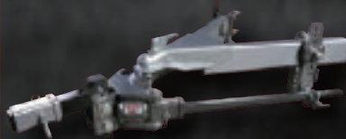
■ Weight Distribution Center-Line Towing System with Active Sway Control
