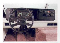
The instrument pod tilts upward for easy service access. Large, easy to use rocker switch controls are at your fingertips. Emergency start solenoid, intermittent wipers and a radio power-selection switch come with every Sunrise. A master battery disconnect switch for care-free coach storage is optional.
