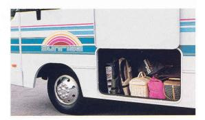
Large exterior locking storage bays are made of steel, have insulated, radius-cornered doors and include high-quality, automotive-type weather seals.
