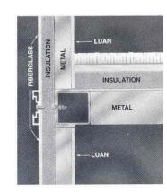
The Sunrise floor to wall joint has a custom extrusion that locks the two pieces in place. This design has a great advantage over the competition because the weight of the floor is supported by this joint, rather than by screws that simply attach the two pieces together.
