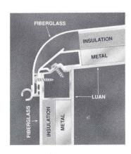
Sunrise's crowned fiberglass roof wraps over the joint onto the sidewall for a smooth, attractive fit. Our exclusive locking joint system joins roof and sidewalls, providing maximum strength and stability.
