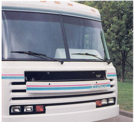
The stylish, aerodynamic front end is as functional as it is beautiful with extra-large driver and passenger side windows, recessed clearance lights and a single, full-width hood for easy access to the engine compartment. Quad headlights and large turn signals add style and safety. Large wipers improve wet weather vision and feature a single powerful motor.
