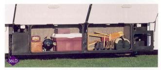
For greater strength, ease of use, and beauty, Itasca Horizon is equipped with new frameless, fully insulated, flat panel compartment doors that feature gas spring supports and single paddle latches. The front slideout features our revolutionary <a href="STOREMORE">STOREMORE</a>\* Hydraulic Slideout System. For easier loading and unloading, lights are located within the StoreMore exterior storage compartments.
