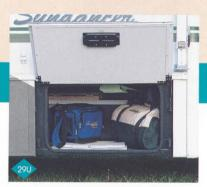
Our pass-through storage compartments feature fully hinged and insulated belt-line storage doors with a single handle latch and gas struts for easy one-handed operation.
