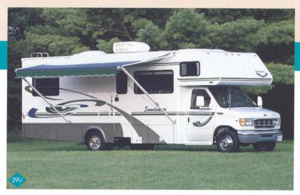
Sundancer's array of exterior features is impressive: fiberglass running boards, available stainless steel wheel liners, valance paint, and an available awning. Our crowned, one-piece fiberglass roof offers more than increased strength and durability. The crowned exterior roof sheds water into the rain gutter that is extruded as part of the awning rails on both sides of the coach.
