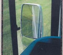
Electronic remote control mirrors feature large flat and convex surfaces and are strategically positioned to provide increased visibility and safety. Electric defrost helps keep mirrors clear.
