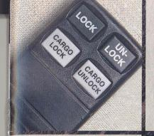
A keyless entry remote locks and unlocks the entry and compartment doors. The KeyOne™ system also allows these doors to be opened with a single, double-bitted key.
