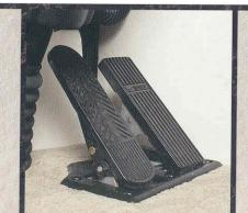
Full anti-lock air brakes provide impressive stopping power. The treadle foot brake pedal is mounted solidly to the steel cab deck to provide maximum brake pedal feel and control. Ulti-Bay is Winnebago Industries' exclusive monocoque chassis design that provides abundant mid-coach storage, impressive driving and handling performance, as well as 10,000 pounds of towing capacity.+
