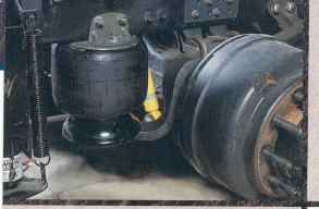
The air suspension system utilizes a single, large air bag over each wheel which provides improved suspension and ride characteristics over less advanced multi-bag systems. Each air spring is placed in a wide-track stance just inside the rear wheel. This position improves stability and helps protect the air springs from road debris that could be kicked up by the tires.
