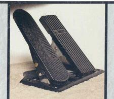
Anti-lock air brakes deliver impressive stopping power. The treadle-style foot pedal is mounted securely to the steel cab deck for maximum feel and braking control.
