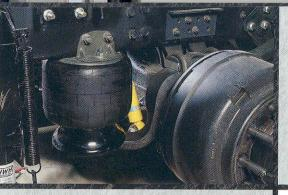
The air suspension system utilizes a single, large air bag inboard of each wheel assembly which provides improved suspension and ride characteristics over less advanced multi-bag systems. Air springs are placed in a wide-track stance just inside the wheels. This position improves stability and helps protect the air springs from road debris that could be kicked up by the tires.
