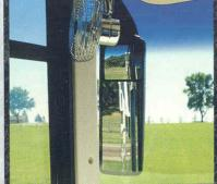
The large, top-mounted exterior mirrors include both flat and convex surfaces and are positioned to reduce road vibrations and give you a full view of the road. Electric defrost keeps the mirrors free from snow and ice during the winter months.
