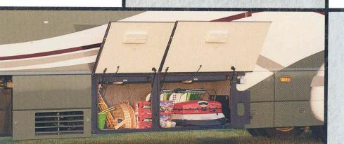
StoreMore® is storage the way it is supposed to be. With the StoreMore Slideout System, the front exterior storage bays actually move with the slideroom for easy access even with the slideroom extended. Storage bays are large enough to accommodate oversized items and storage bay doors feature gas struts and a single-paddle latch for easy, one-handed operation.
