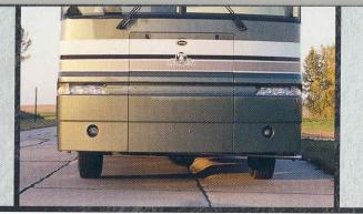
The independent front suspension (IFS) on the Freedom can make any road seem like a newly paved highway. Some luxury coaches still use straight axle technology that transfers road forces from wheel to wheel — reminiscent of heavy trucks. IFS, however, provides greater lateral stability, eliminates bump steer and lets each wheel move independently through its range of motion. Each tire maintains better contact with the road and you get a smooth ride comparable to that of a luxury sedan.
