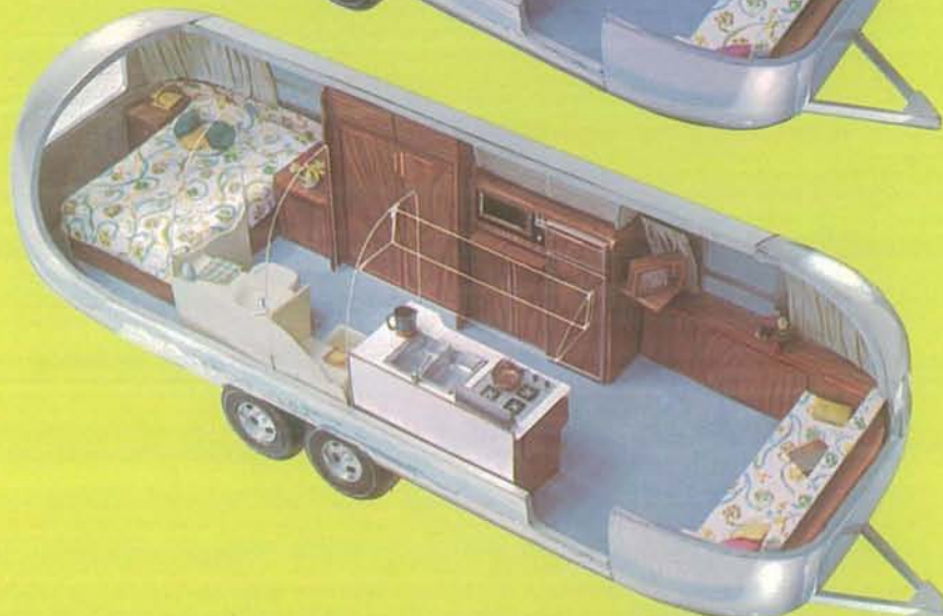
29 FT. AMBASSADOR DOUBLE CENTER BATH (International Land Yacht) Hitch Wt. 635 lbs. Total Wt. 4765 lbs.
