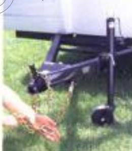
not interfere with tow vehicle's tailgate or rear mounted spare tire. (Highlander Series features center mount jack with detachable wheel.) Safety lock chains provide a positive locking connection between the trailer and tow vehicle.
