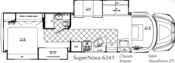
Length 36'6" Height W/AC 12' 7" Width 101" Interior Height 83" Interior Width 96" Fresh Water 150 gal.
