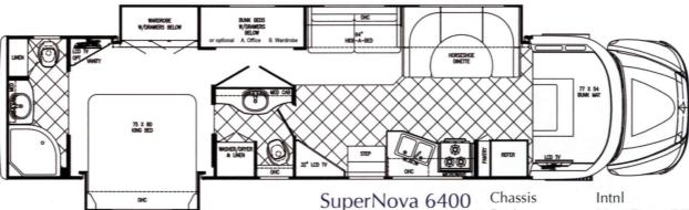
Length 40" Height W/AC 12' 7" Width 101" Interior Height 83" Interior Width 96" Fresh Water 150 gal. Grey/Black Water (2) 52 gal. Water Heater 12 gal. LP Gas Tank 64 lbs. Furnace BTU's 35,000 Chassis Intnl
