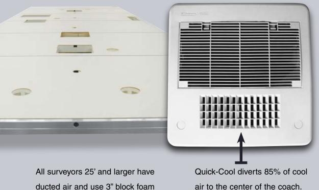
ducted air and use 3" block foam insulation (R-11). All surveyors have a walkable roof and rear ladder option.
