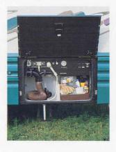
Swivel holding tank drain valves, wash station, black water tank flush system, sewer hose and cover, telephone and cable TV inputs, and 90 degree fresh water fill with tank fill diverter valve are conveniently located in all service centers.
